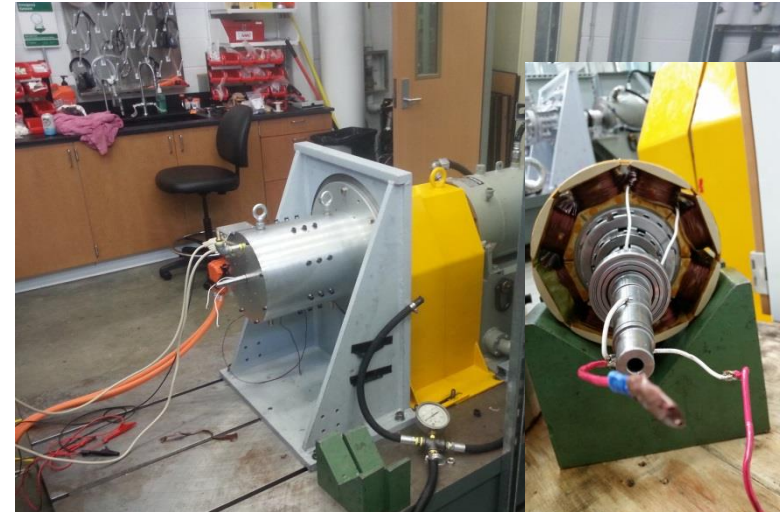
Wound Field Traction Machine
